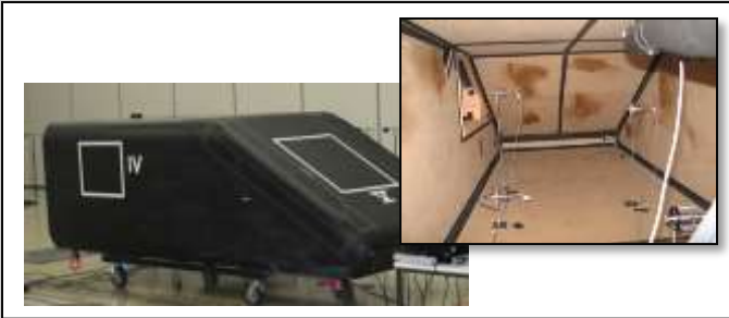
Measurement of SPL inside SAE body for Omnisource excitation
