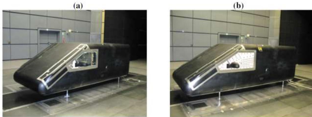
Figure 14. Wind-tunnel test: (a) glass module, (b) sensor module
